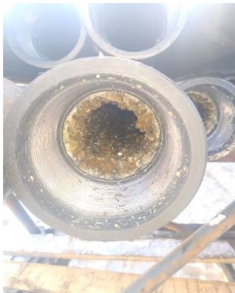
Figure 3. Sediments (calcite) in downhole equipment
